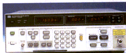
5. The HP 8970B NF meter has long been a precision tool for simultaneously characterizing the NF and gain of low-noise devices.
